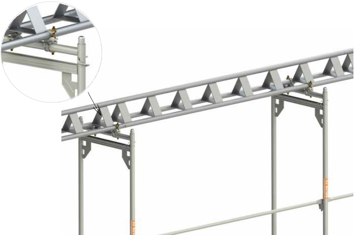
Fig. 65. Mounting the roof guide rail and the rail connector with the frame.
