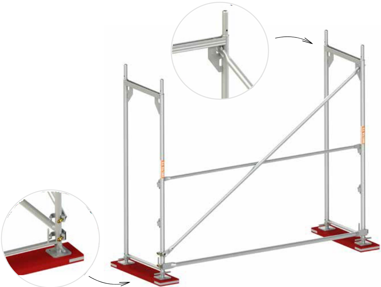
Fig. 4. Installation of the first vertical frames, handrails and diagonal brace in the base bay.
