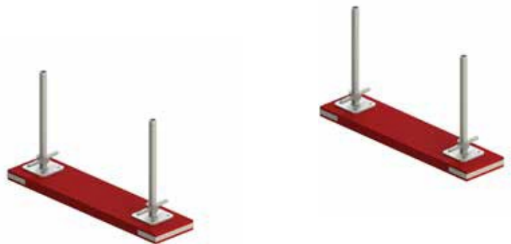
Fig. 2a. Foundation of scaffolding on wooden sleepers.
