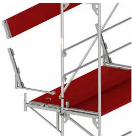
Fig. 17a. Installation of protective canopies in accordance with the PN-EN 12811-4:2014-02 standard.
