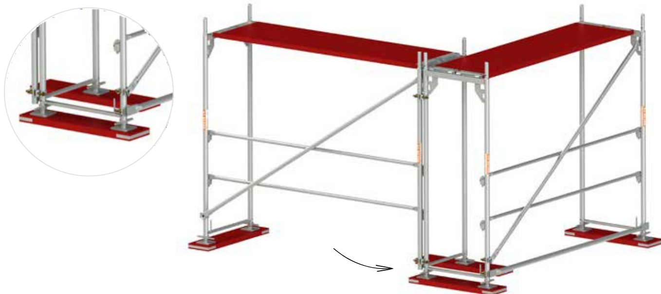
Fig. 29b. Assembly of corners with rotary joints.
